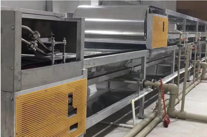
Double belt cooler for resin
